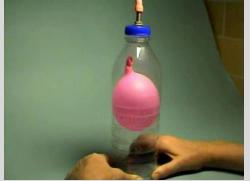
The over pressure in the bottle, caused by velocipede tire-pump, causes reduction in volume of the balloon.
