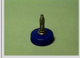
Overpressure in the plastics bottles in all experiments is made out by hand-pressing or by a small velocipede tire-pump.
