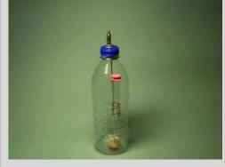
**•** The membrane under the influence of pressure is bent into the test tube.
