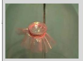
The rubber and plastic membranes simulate behaviour of ear-drum during swimming, bathing and diving. Water in ear (ear canal) pushes on ear-drum similarly as air on membranes in the case of our experiment. The result of this pressure is deformation of the eardrum and in the case of high pressure (overpressure) rupture of the ear-drum.
