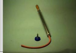
Experimental kit is easy to be built. For time reasons, it is advisable to prepare it before experimentation. From a security point of view it is necessary to use protective goggles or face shield. Plastic bottle is designed to withstand high pressure, yet we permit students to pump only a few times. It must be checked proper and secure closure of the bottle.
