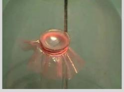
▶ If overpressure in the bottle is sufficiently great, the plastic membrane ruptures.
