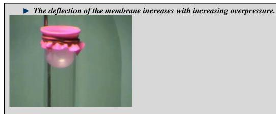
Replace the rubber membrane with a thin plastic membrane.
