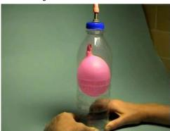
▶ The over pressure in the bottle, caused by velocipede tire-pump, causes reduction in volume of the balloon.
